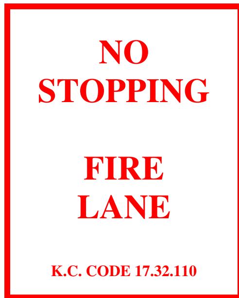
Figure D103.6 Fire Lane Sign
